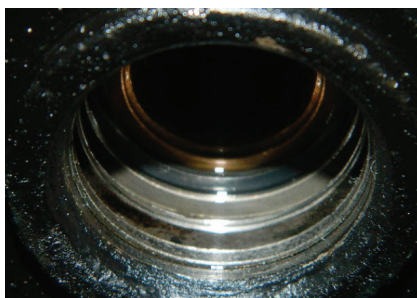
Oil leak on Exhaust side casing
