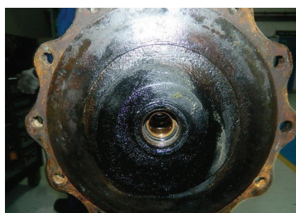
Oil leak on Exhaust side casing
