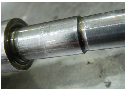
Scoring mark on rotor shaft
